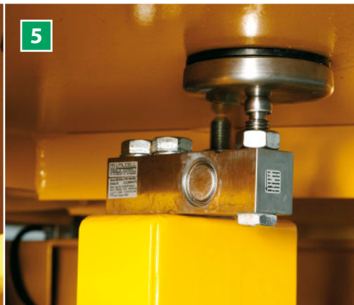
5 Load cells The pan mixer is placed on three 11.025 pound electronic load cells with an accuracy of +/- 0.5%.
