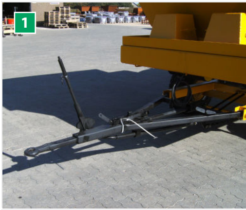
1 Bogie trailer Joint triple-axle bogie in a welded steel frame with a turnable front axle. The draw hook can be dismantled and thus helps to prevent theft. The trailer also has a parking brake.
