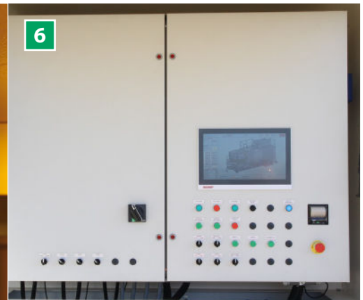
6 Control system Possibility of manual, semi-automatic, and automatic operation and PC interface. No previous knowledge required and can be delivered with the language version desired. Stores 50 recipes. Dosing accuracy: +/- 0.5 - 2%.
