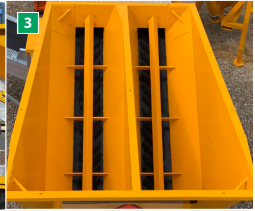
3 Hoppers Two integrated twin hoppers for 2 x 2 types of aggregate. Each hopper holds 2 x 2.14 m 3 . Made in all-welded steel plate with reinforced corners. 2 x 2 separate feed belts for the dosing of aggregates.
